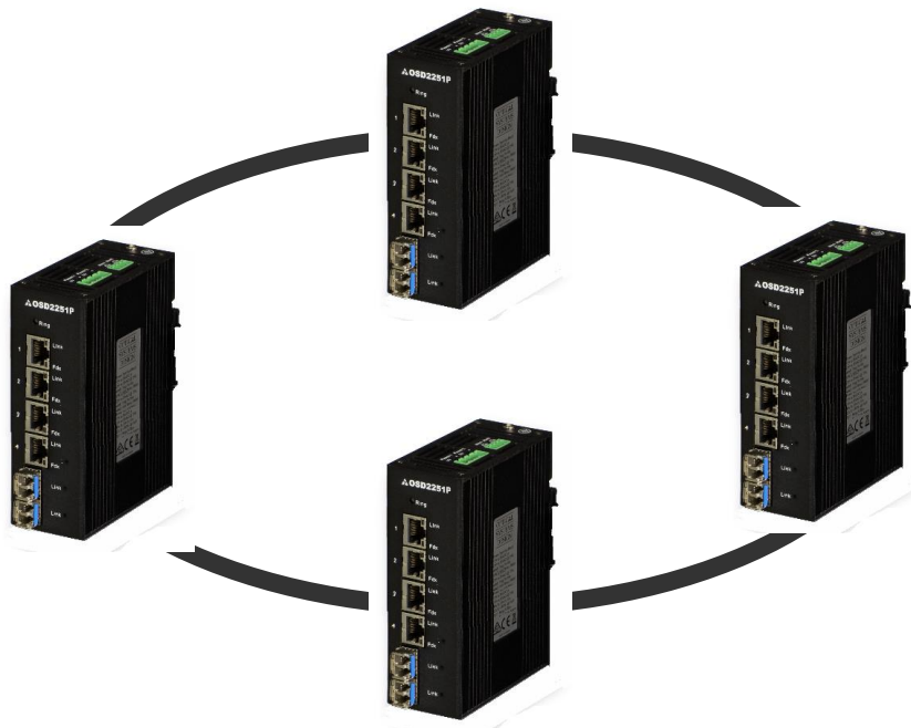
FIGURE 14: REDUNDANT RING CONFIGURATION
