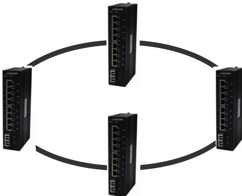
FIGURE 14: REDUNDANT RING CONFIGURATION
