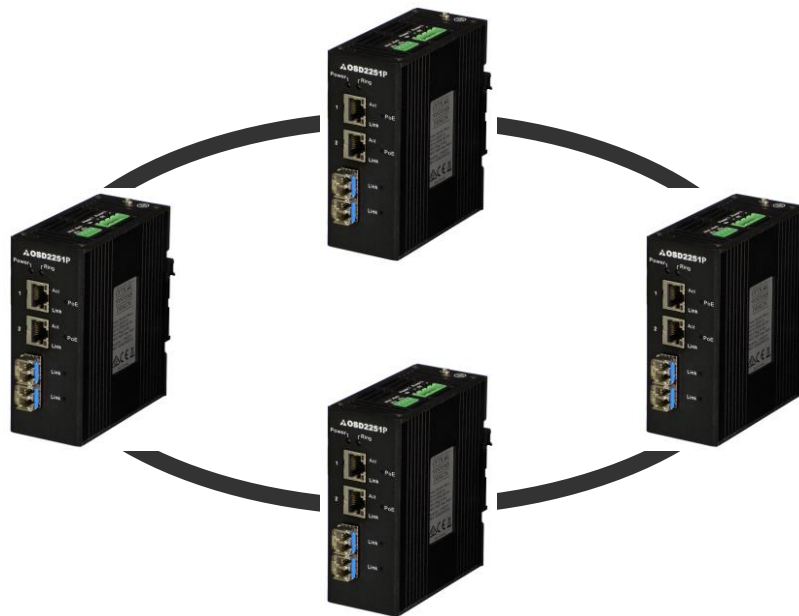
FIGURE 14: REDUNDANT RING CONFIGURATION
