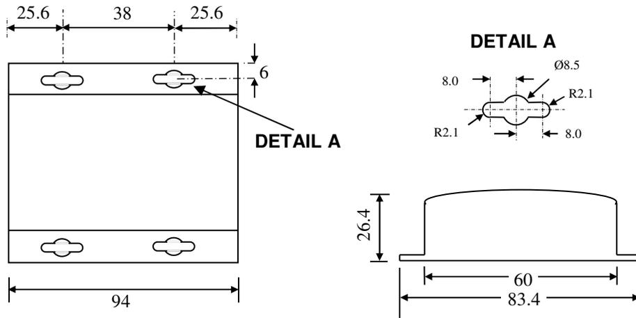
FIGURE 3: OSD2167M MOUNTING DIMENSIONS
