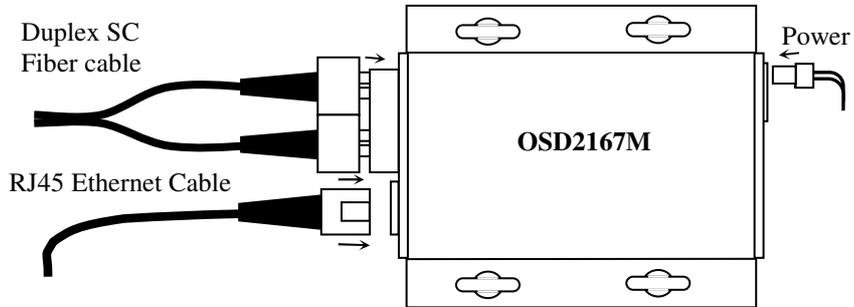
FIGURE 7: BASIC CONNECTIONS
