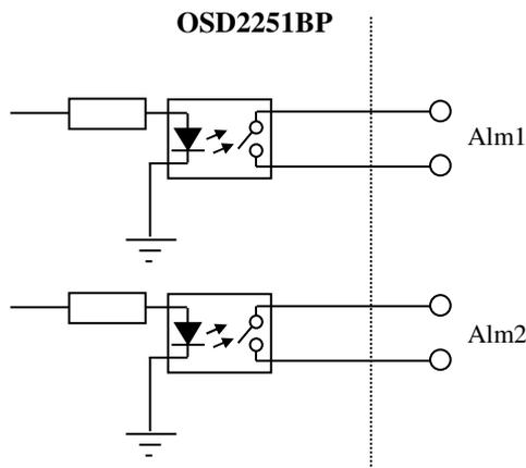
FIGURE 6: CONTACT CLOSURE OUTPUT
