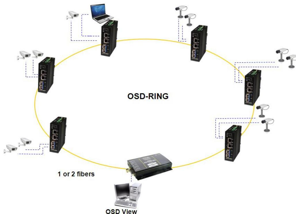
FIGURE 1: TYPICAL RING CONFIGURATION
