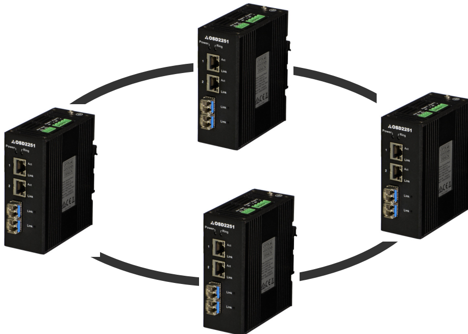
FIGURE 13: REDUNDANT RING CONFIGURATION
