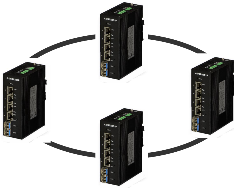
FIGURE 14: REDUNDANT RING CONFIGURATION
