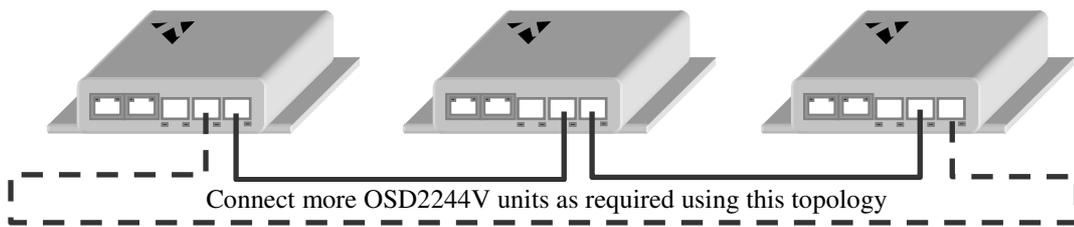
FIGURE 13: REDUNDANT RING CONNECTION
