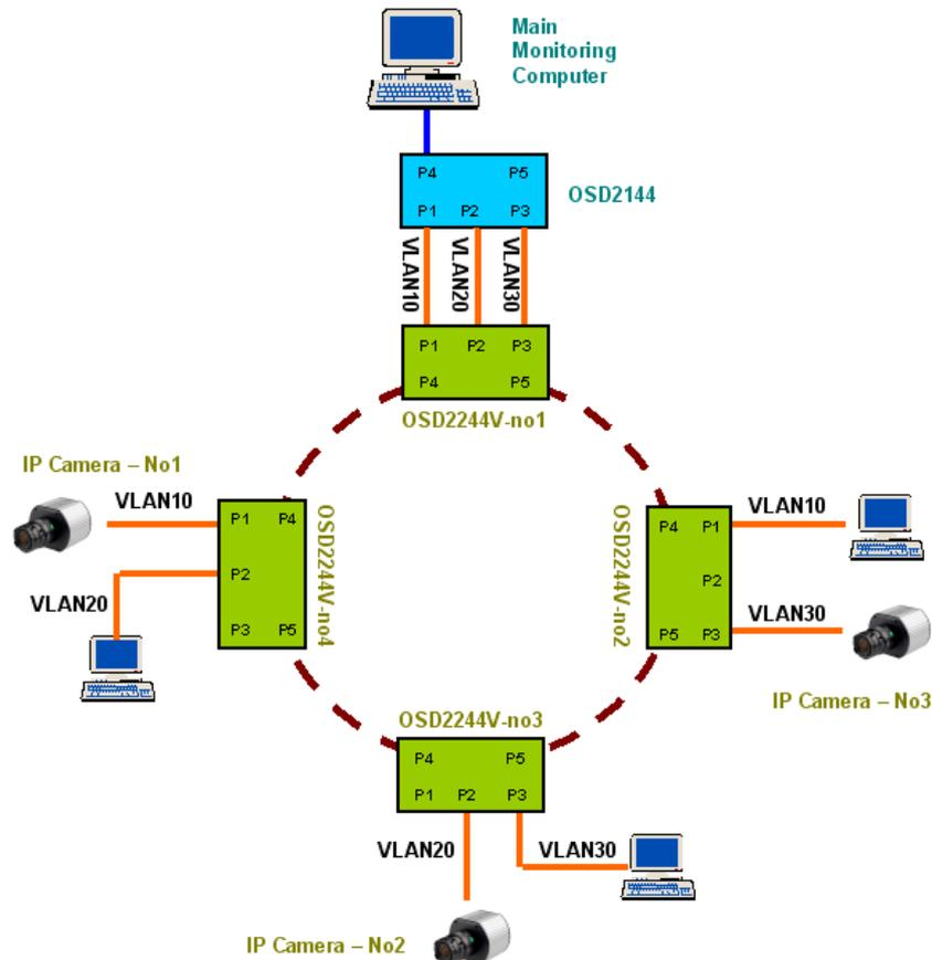
Four OSD2244V operating with one OSD2144 (unmanaged switch) to access multiple cameras on one PC
