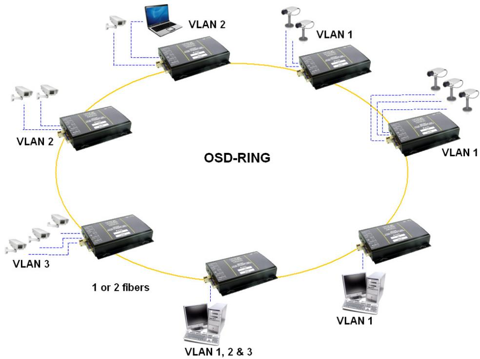
FIGURE 1: OSD2244V TYPICAL RING CONFIGURATION
