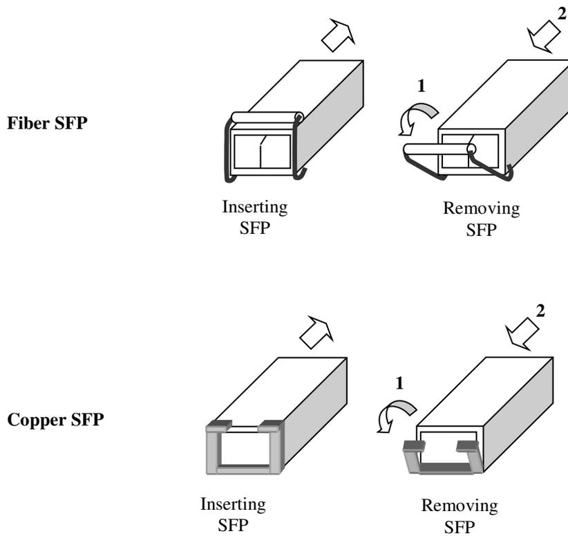
FIGURE 11: FITTING/REMOVING SFP CONNECTORS
