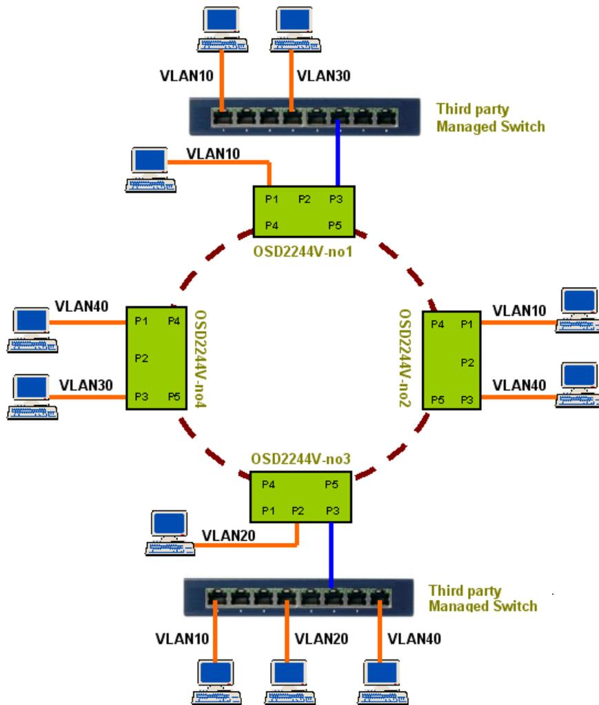
Four OSD2244V operating with two third-party managed switches to build an IEEE802.1Q VLAN
