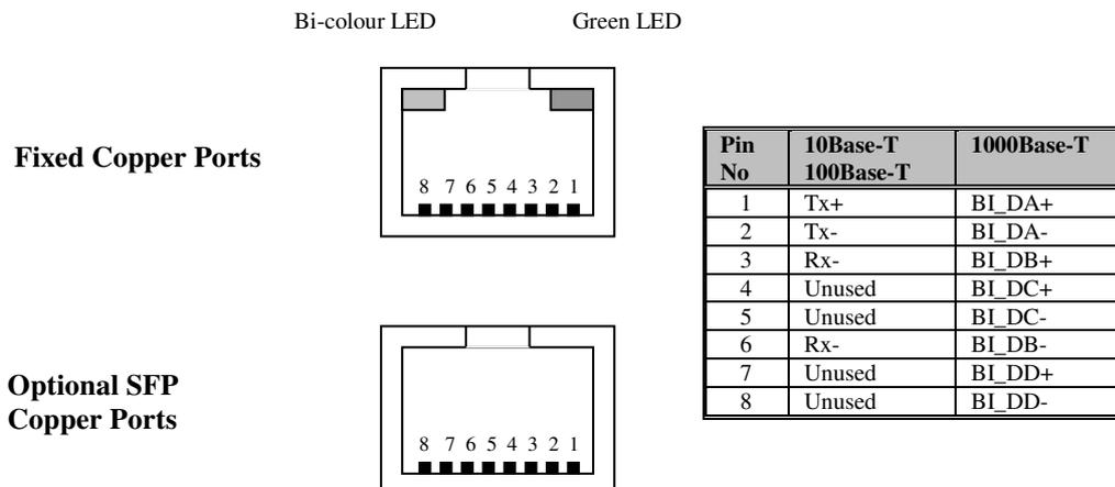
FIGURE 5: FIXED 10/100/1000BASE-T ETHERNET RJ45 CONNECTORS
