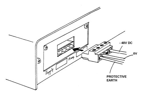
Figure 1. -48VDC Power Supply Connection
