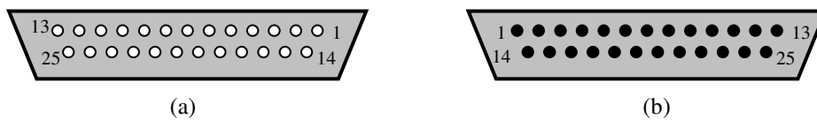
FIGURE 2: D CONNECTOR PINOUT CONFIGURATION. (a) Female Connector, (b) Male Connector
